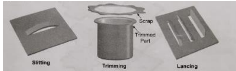
Figure 1.21: Slitting, Trimming and Lancing
