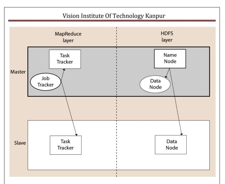
Hadoop Distributed File System : The Hadoop Distributed File System (HDFS) is a distributed file system for Hadoop. It contains a master/slave architecture. This architecture consist of a single NameNode performs the role of master, and multiple DataNodes performs the role of a slave.
